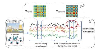
Figure 1: (a) Unsupervised anomaly detection and diagnosis in multivariate time series data. (b) Different system signature matrices between normal and abnormal periods.
