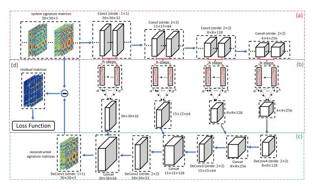
Figure 2: Framework of the proposed model: (a) Signature matrices encoding via fully convolutional neural networks. (b) Temporal patterns modeling by attention based convolutional LSTM networks. (c) Signature matrices decoding via deconvolutional neural networks. (d) Loss function.
